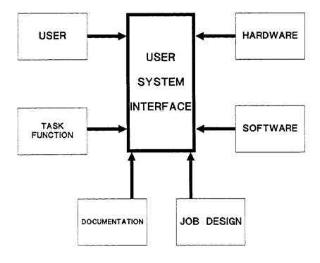
Figure 2. Elements of the User-Computer Interface
